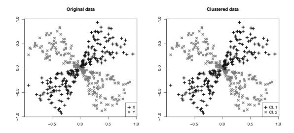
Figure 1: Left: Hourglass data set used in the first multivariate experiment, collecting N=400 points subdivided into family X (K=200 points, marked by +) and family Y (K=200 points, marked by ×). Right: Outcome of clustering via Max-Swap algorithm.
