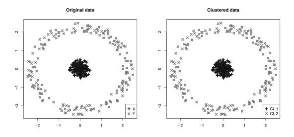
Figure 2: Bull's eye data set used in the second multivariate experiment, collecting N=400 points subdivided into family X (K=200 points, marked by +) and family Y (K=200 points, marked by ×). Right: Outcome of clustering via Max-Swap algorithm.
