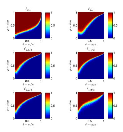
Figure 8: Phase diagram study of  $\ell_{p,q}$  regularization of group sparse optimization. Blue denotes perfect recovery in all experiments, and red denotes failure for all experiments.
